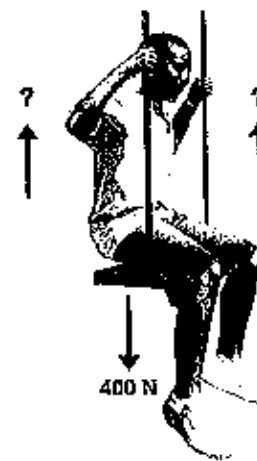
Figure 5.21: What is the tension force in each rope holding up the swing?
